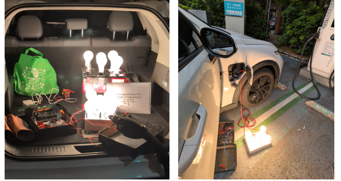
(a) Unauthorized autocharge at a public station. (b) Unauthorized forced discharge via rogue EVSE setup.
